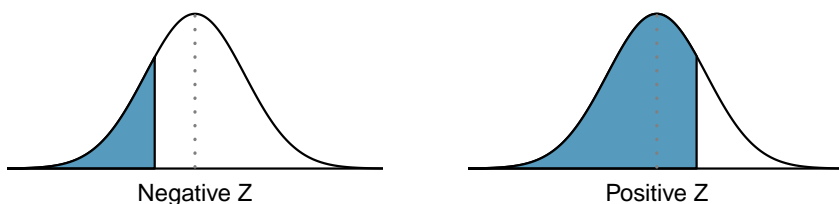
Figure C.2: The area to the left of Z represents the percentile of the observation.
